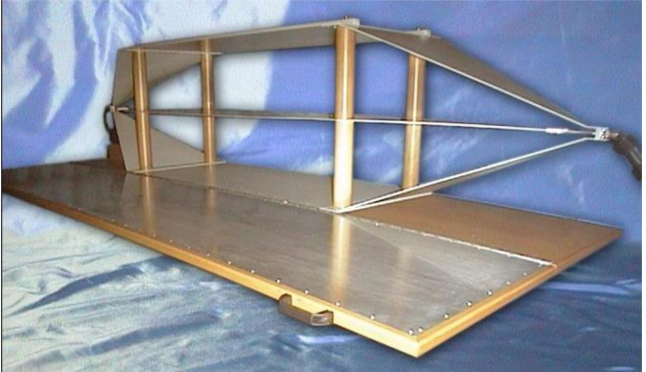
The triplate is an OPEN TEM cell of widespread use by the automotive community. The reference specification, SAE J1113-25 of September 1995, revised in March 1999, gives the instructions on how to build and test the device.
