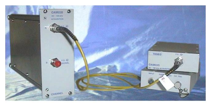
**TESEO** DC and low frequency plug-in systems and remote satellites are fiber optic communication links for the transmission of analog signals, including DC, in hostile environments subjected to electromagnetic interferences, noises, or characterized by the presence of high voltages.
